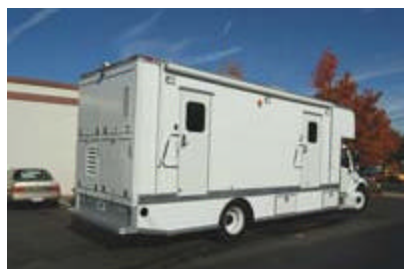
Larger, general purpose mobile lab can be used for chemical, biological, nuclear, radiological, and explosives testing in the field. Labs are available with all
