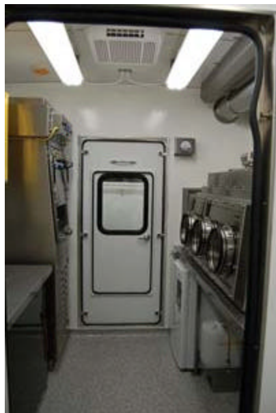
Sample preparation capabilities in BSL-3 type secure mobile lab can be certified for use in testing bio-hazards in the field. Photo: E-N-G. Click here to enlarge.
