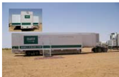
One of the first trailer modules is shown in Saudi Arabia with pop-out side panels extended, more than doubling the interior floor space of the mobile lab. Photo: Facilities Solutions Group, Gulf Care Intl. Click here to enlarge.
